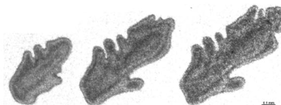
Figure 2: X-Ray Topographs recorded in situ at ESRF during solidification of an aluminum alloy and showing successive stages of the growth of a dendrite. (H. Nguyen Thi, B. Bilia, T. Schenk et al.)
