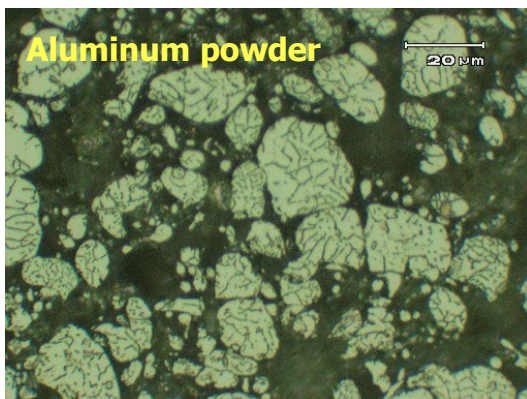
Figure 5: Cross sections of (a) aluminum powder particles and (b) bulk aluminum consolidated from the powder by UPC at 573 K under 100 MPa [6].
