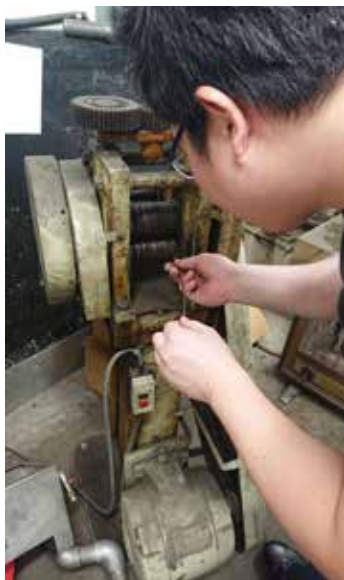
▲Metal forming by roll grooving method
