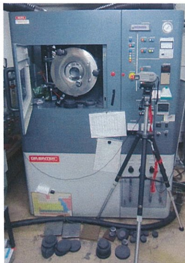
Fig. 3 SPS apparatus DR.SINTER (Fuji Denpa) in Cooperative Research and Development Center for Advanced Materials / IMR.
