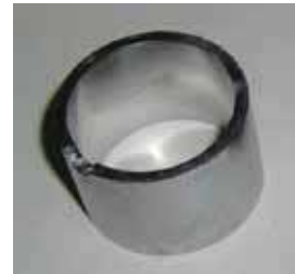
Fig.6. View of original Re after-heater.
