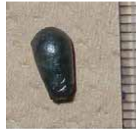
Fig.7. As grown Lu_2O_3 crystal. Scale is in mm.
