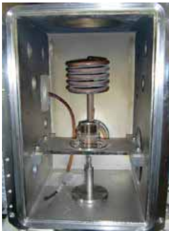
Fig.2. View of the actual \mu -PD systems with quartz tube (top) and chamber (bottom) designs.
