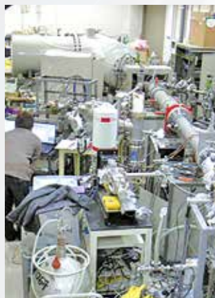
1.7MV tandem accelerator for ion-beam analysis and materials modification
