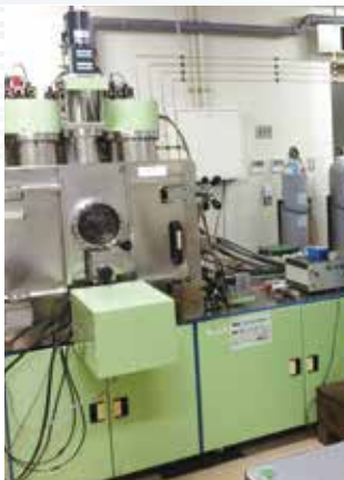
Multi-Target Reactive Sputtering (Ion Beam Sputtering)
