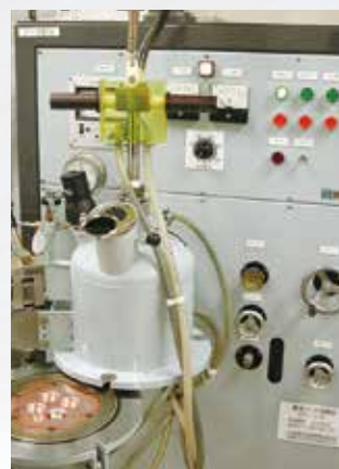
Conventional type arc-melting furnace
