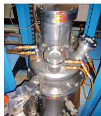
3 Crystal Pulling Apparatus of the Transverse Applied Magnetic Field Type
